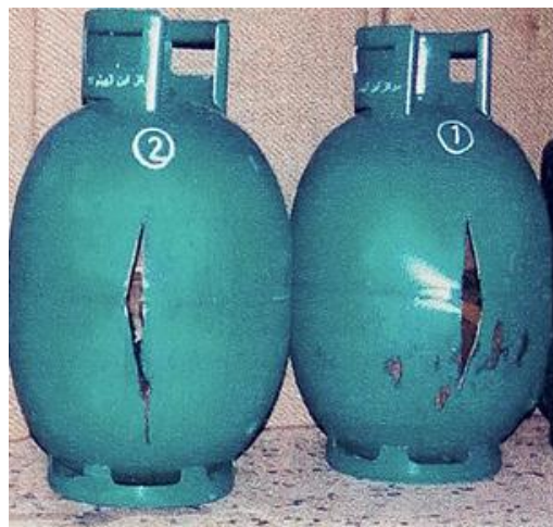
Fig.3. Failure Locations of the cylinders.
