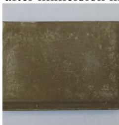
Figure 4 photo for Aluminum alloy after immersion in Desalination water
